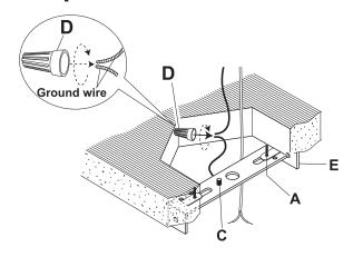
Attach the ground wire from the fixture to the ground junction box wire from the ceiling box (usually green), fasten each together with a Plastic Wire Connector (D) and wrap the connection with electrical tape (not included). If your ceiling box does not have a ground wire, insert the Green Ground Screw (C) into the Mounting Plate (E) facing down, and wrap the fixture's ground wire around the Ground Screw (C).
