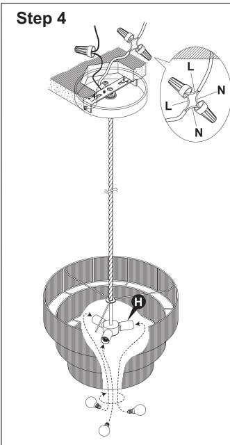
Attach the bulbs (not included) to the Sockets (H) then turn until tightened.
