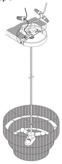
The Light Fixture installation is now complete. Turn power back on at the main electric circuit supply and check the light for operation.
