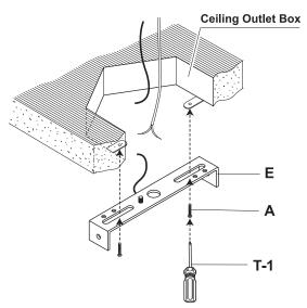
NOTE: Turn off main electrical power before beginning. Attach Mounting Plate (E) to the Ceiling Outlet Box using Mounting Screws (A) tighten with a Screwdriver (T-1) (not included).
